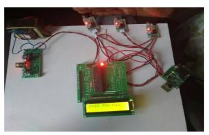
[3]Receiver consists of pic controller, power supply,LCD and ZigBee communication protocol.
